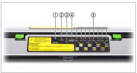
Figure 33: Button and indicators on memory board
